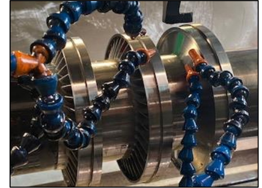
Turbine Rotor First and 2 nd Stage Completed
