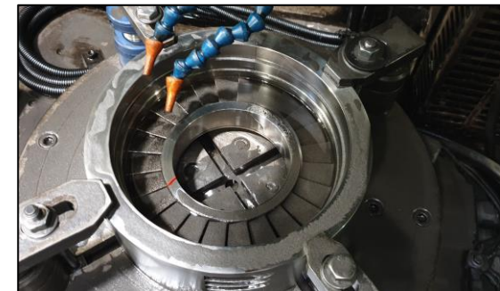
Turbine Stator Nozzle Machining
