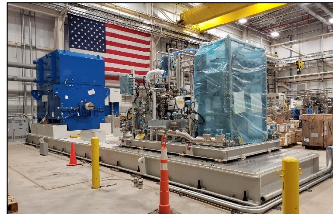
Turbine Skid in the High Bay with Generator in place and Bypass Compressor Sub-Skid
