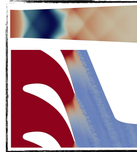
CONDENSING WET STEAM (LES) [6]
