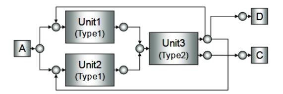
The superstructure can easily be created in the Process Simulation Software, by using "split" modules (concept of "switch")
