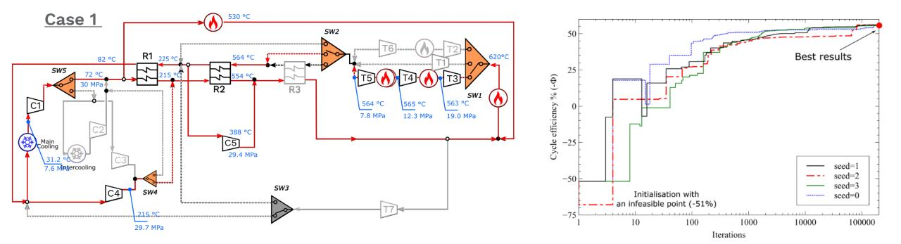
$\eta$  = 51 % Double reheating-double recompressionpreheating cycle
