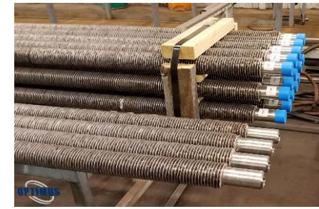
IN740H tubing with 304S fins
