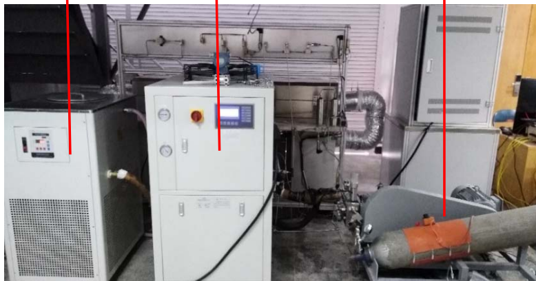
Control Valve Back pressure Valve Test section Cooler Condenser Pump and Gas bottle
