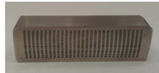
In house welding sample of a diffusion-bonded micro heat exchanger
